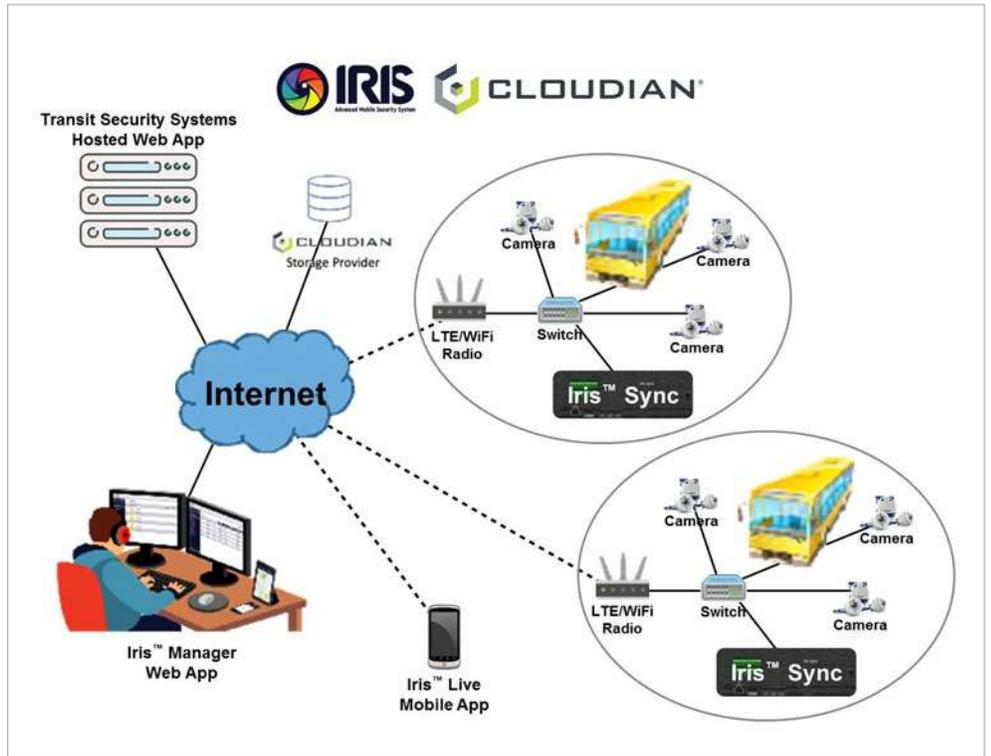
Clouidian object storage provides the central repository for surveillance video data. Rich metadata tagging allows personnel to search clips by time, geographic location, vehicle ID, and other parameters for rapid data discovery.
